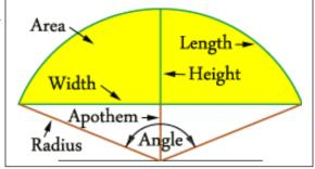
To measure the Height in the field, simply pull a tape or straight line along the full width then measure the height from straight line to backside of panel.
